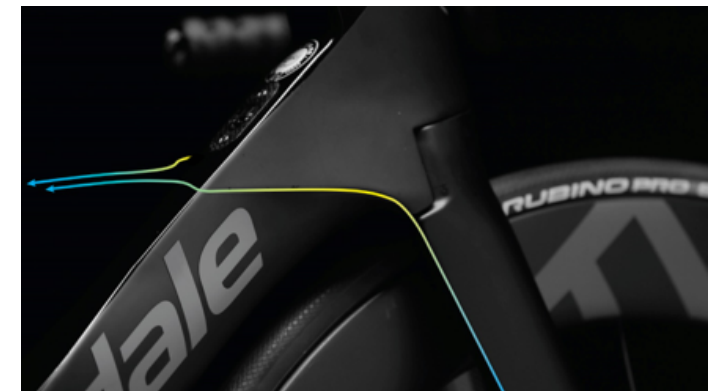
Figure 18 - Flow moving up the fork crown is redirected downstream by the chine.
