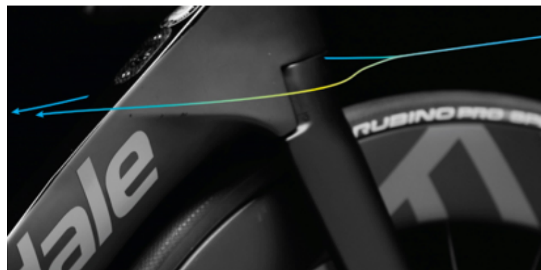
Figure 17 - A cross section of continuous airfoil over the fork crown.
