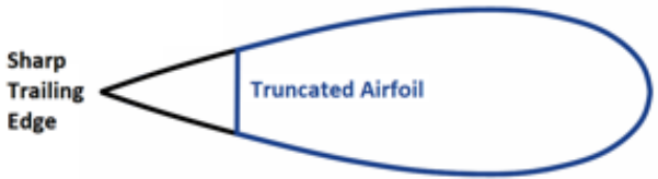
Figure 15 - Airfoil with sharp trailing edge (black) and truncated airfoil created from same airfoil (blue).
